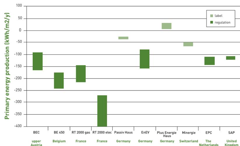
Primary energy production levels -regulations and labels- (including heating, domestic hot water, ventilation and lighting) in mid European climates (negative values correspond to a consumption)
