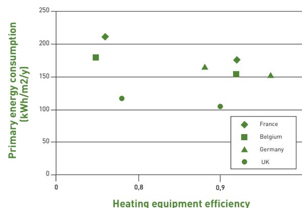
The main parameter is the boiler efficiency. The energy consumption decreases by around 2.3 kWh/m<sup>2</sup>/y if the efficiency increases by 1% (e.g. from 75% to 76%).
